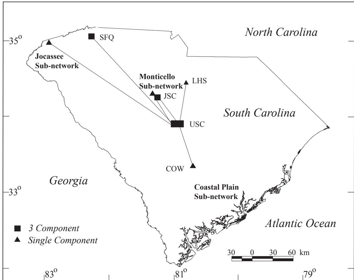
□ □ Figure 13. □ Telemetry routes for seismic data transmitted to USC.
