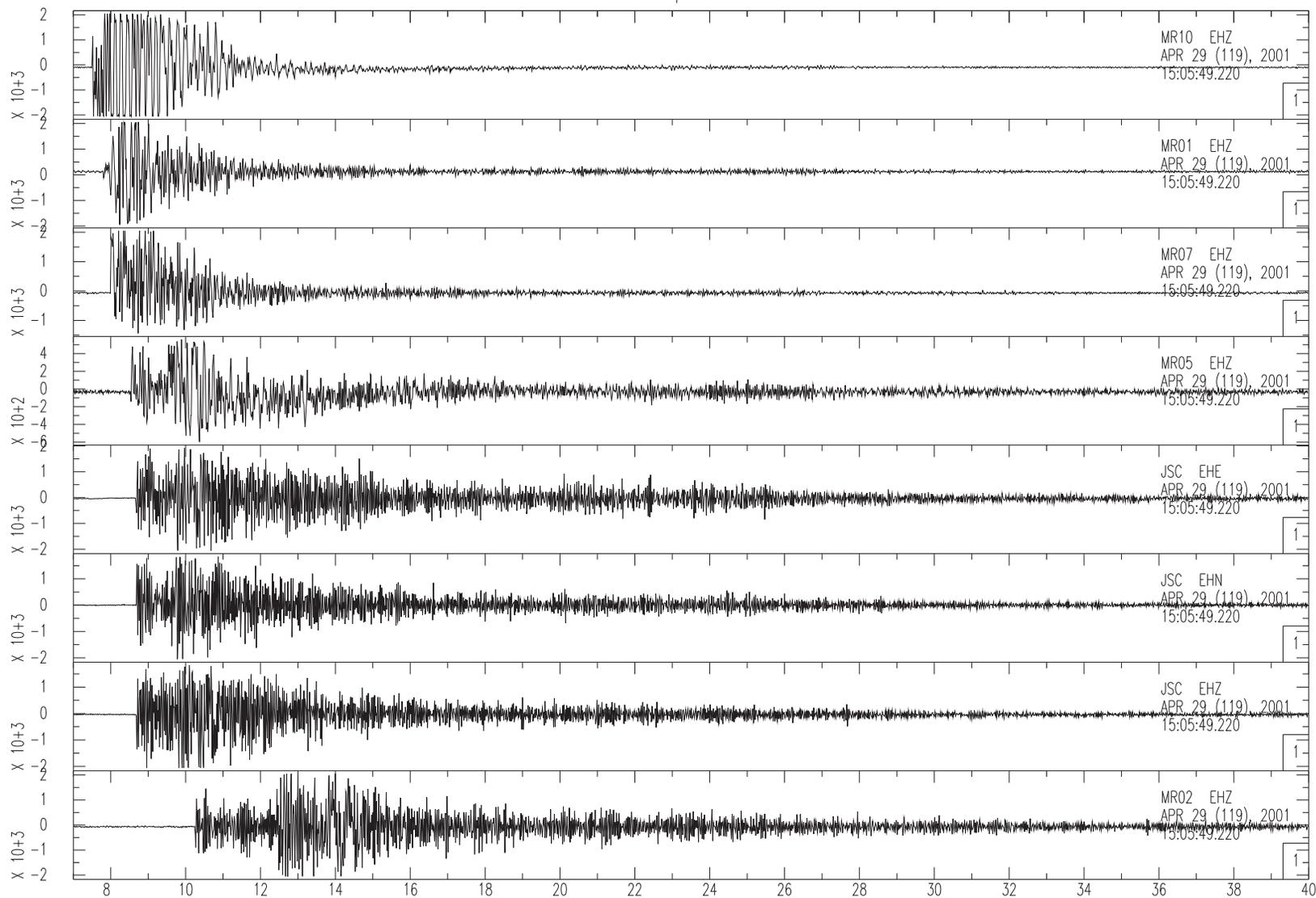
Figure 7c.  Digital playback of a ML 1.8 Monticello Reservoir earthquake on April 29, 2001.
