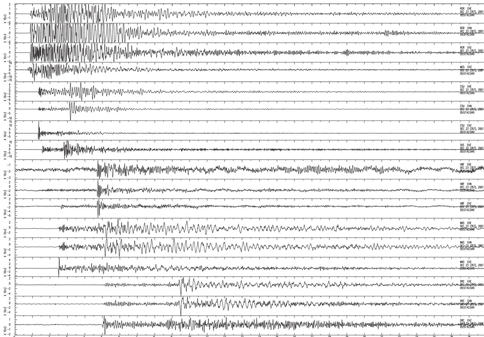
□ Figure 7a. □ Digital playback of a ML2.8 earthquake in the MPSSZ during 2001.
