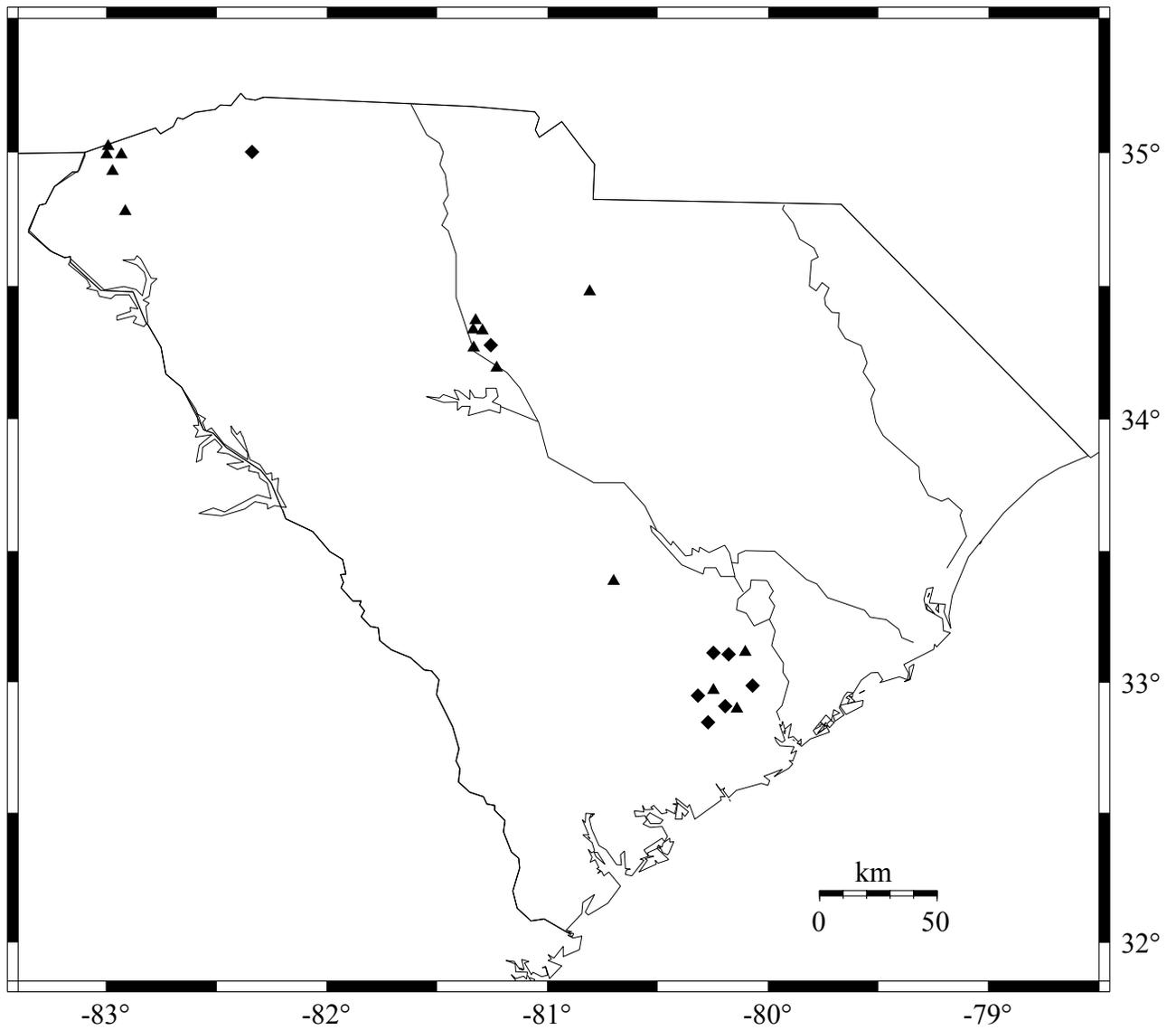
Figure 1. □ □ Distribution of stations/subnets of the South Carolina Seismic Network during 2001. Triangles represent single component stations while diamonds signify three component stations.
