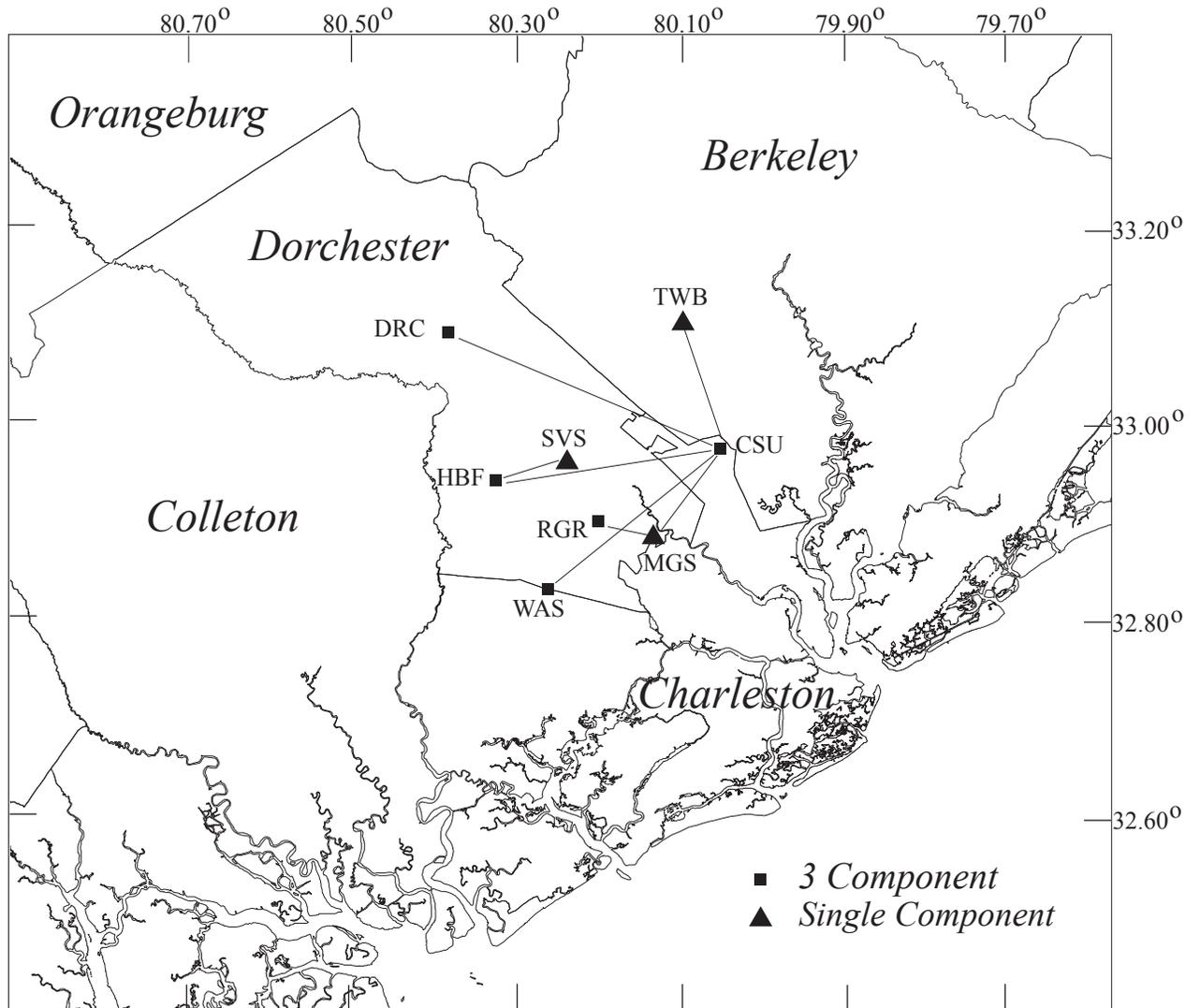
Figure 14. □ Telemetry routes for seismic data to Charleston Southern University.
