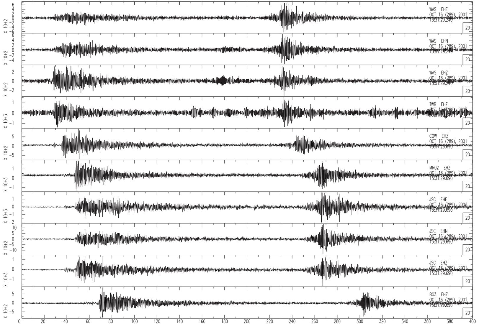
□ □ Figure 7d. □ □ Digital playback of a Mw 5.7 earthquake near Puerto Rico on October 16, 2001.
